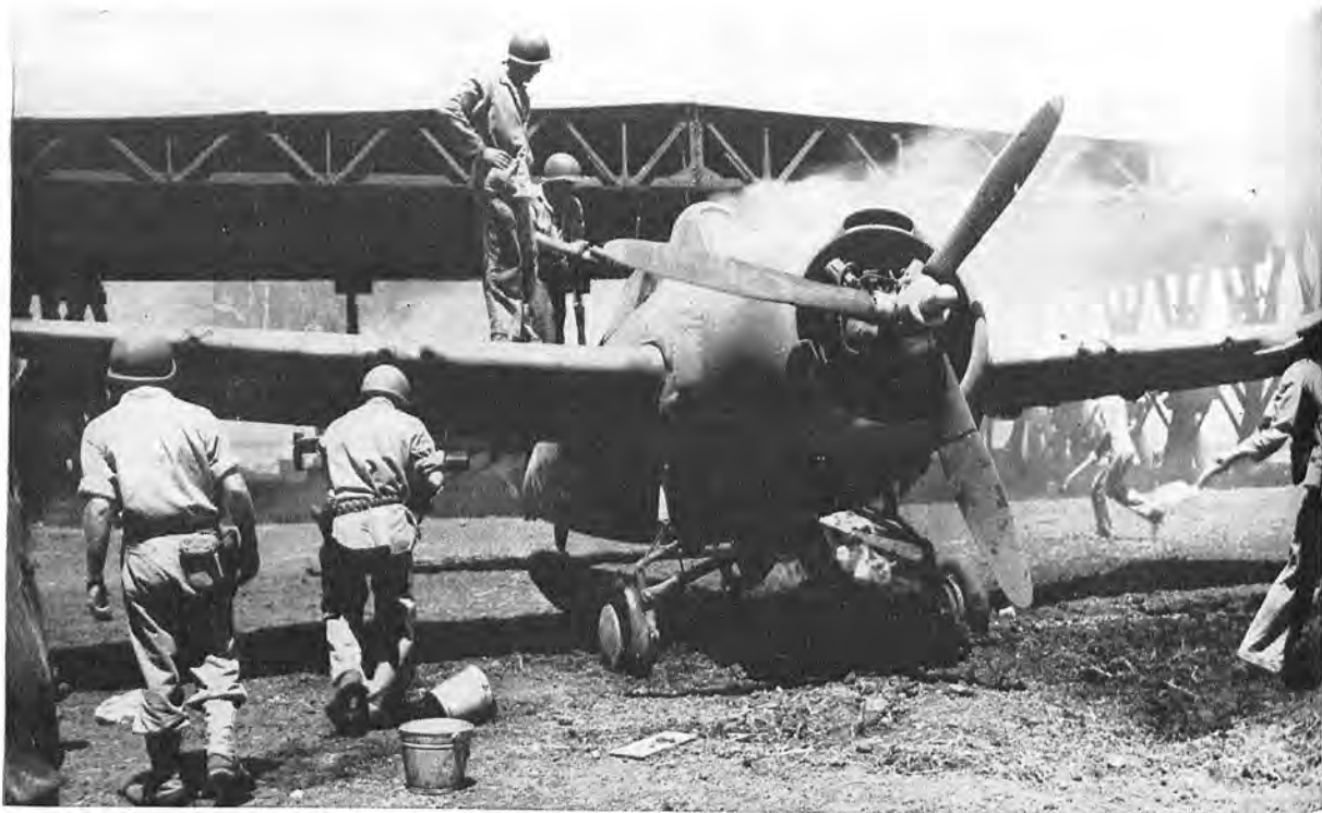
MARINE FIGHTER PLANES fell victim to many mishaps. This MAG-23 F4F-4 is being saved by bucket-brigade methods. Note bullet-pierced propeller-blades.
